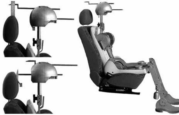
Ryc. 5. Head restraint measurement device (HRMD) według IIHS Fig. 5. Head restraint measurement device (HRMD) according to the IIHS
