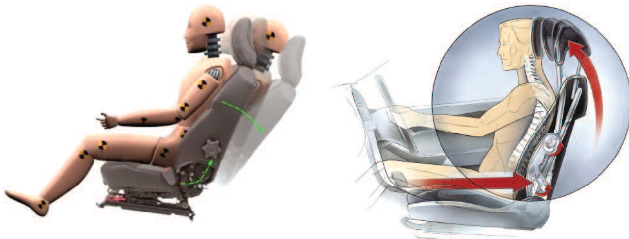
Fig. 3. The principle of the Autoliv Anti-Whiplash Seat (left) and Saab Active SAHR headrest (right).
