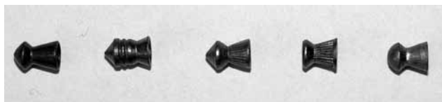
Ryc. 4. Śruty 4,5 mm w kolejności od lewej: Umarex Air Mag, Silver Point, Umarex szpic, Logo Sport, JSB Exact. Fig. 4. 4.5 mm buckshot (from the left): Umarex Air Mag, Silver Point, Umarex cusp, Logo Sport, JSB Exact.
